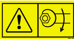
Ensure all nuts & bolts have been tightened prior to operating the machine
