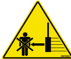
Danger from rotating Prestretcher
